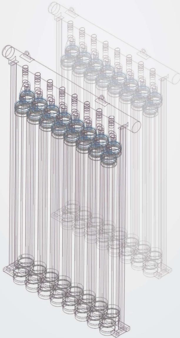
Scinor SMT600 series ultrafiltration modules utilizing our state-of-the-art Thermally Induced Phase Separation (TIPS) PVDF membranes provide the highest permeability, mechanical strength, and chemical tolerance in the industry. These modules are ideal for use in potable water, wastewater, desalination, and industrial applications. The SMT600-S30 retrofits major membrane vendor installations giving end-users a choice when replacing membranes.
